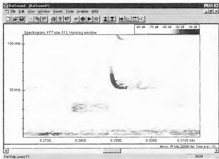
Fig. 2 b). A spectrogram of the same signal as above, but after using a proper anti-aliasing filter.
