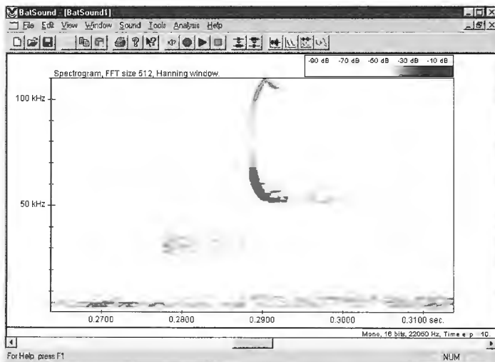
Fig. 2 a). A spectrogram showing a signal with aliasing.
