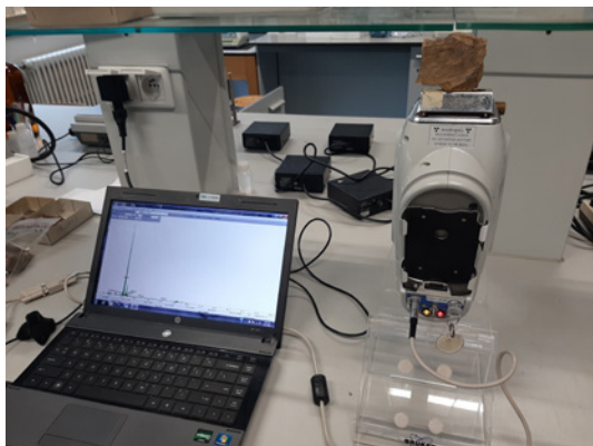
Fig. 5: Setup of the pXRF device at the 'Physico-chemical laboratory' of the geology department of the KU Leuven at Heverlee. The upright position allowed for an easy interchanging of samples.
