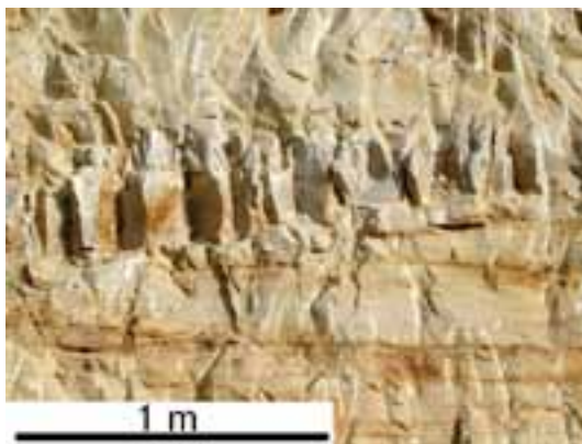
Fig. 6: Closely fractured carbonate-rich bed; fresh roadcut near Mondorf.
