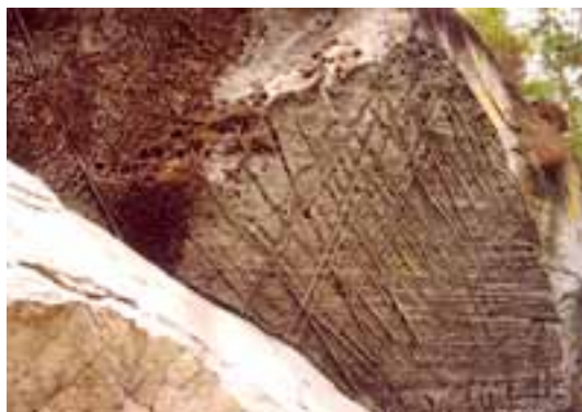
Fig. 2: Two intersecting series of deformation bands at Pod Pětichlappkou locality, Klokočské skály Cliffs. Steeper bands strike NW–SE, moderately inclined bands strike ENE–WSW. View towards ENE. Photo: J. Adamovič.
