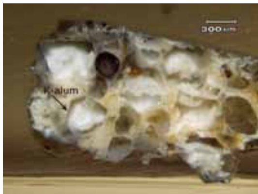
Fig. 1: Crystals of potassium alum KAl(SO_4)_2 \cdot 12H_2O in the pore space of the sandstone from Bohemian Switzerland, cross-section, normal visible light. Photo: J. Schweigstillová.
